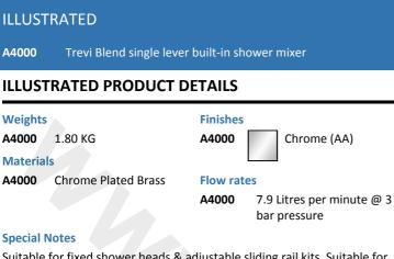
Suitable for fixed shower heads & adjustable sliding rail kits. Suitable for rising or falling supplies. Flow rate 7.9 litres per minute at 0.1 bar. Consideration should be given to safe hot water delivery and the use of an appropriate temperature reduction see A5900AA or Part G for guidence.
